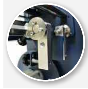
Remove unwanted waste from the edge of the roll
